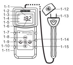
1-1 Buzzer 1-2 % symbol 1-3 Low battery 1-6 Testing value1-7 Warning light1-8 Function key
